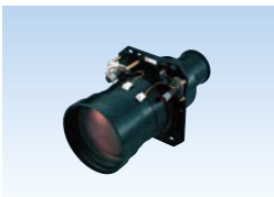
LKRL-Z140 Long Focus Zoom Lens Throw ratio: 3.81:1 to 7.12:1
